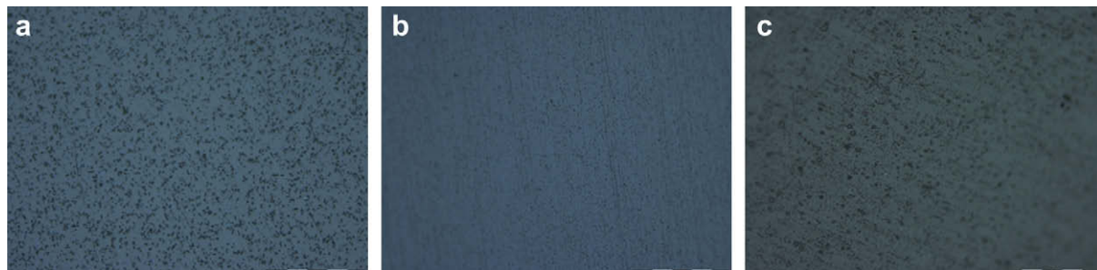
Fig. 2. Light microscopy of 20% wt fully cured samples – a) RTM6 + ZB, b) RTM6 + ZHS, c) RTM6 + ZS.
